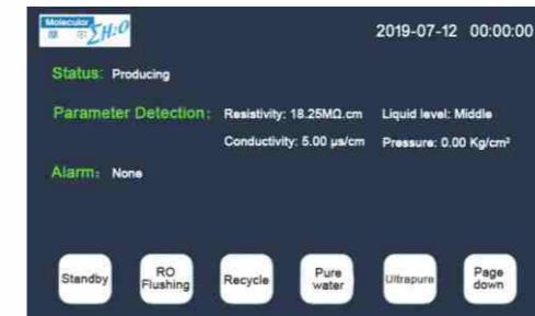
On-line monitoring of working condition and waterquality, pressure, consumablelife span
